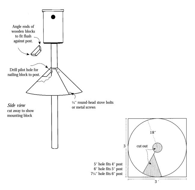
Cut predator guard from a 3′ x 3′piece of 24- or 26-gauge galvanized sheet metal. Join sides with ½″ round-head stove bolts or metal screws. Use angled wooden blocks to nail guard in place.
