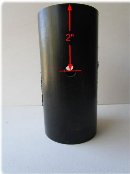
2) Drill a  $\frac{3}{8}$ " hole through the pipe 2" from the notched end. The holes **must be** at a 90 angle to the notches.
